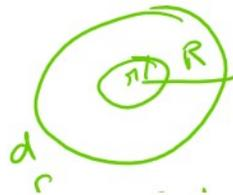
$$\text{Volume} = \pi \int_c^d R(y)^2 dy - \pi \int_c^d r(y)^2 dy$$
