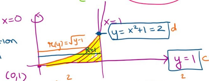
$$\text{Volume} = \pi \int_1^2 1^2 dy - \pi \int_1^2 (y-1) dy$$
